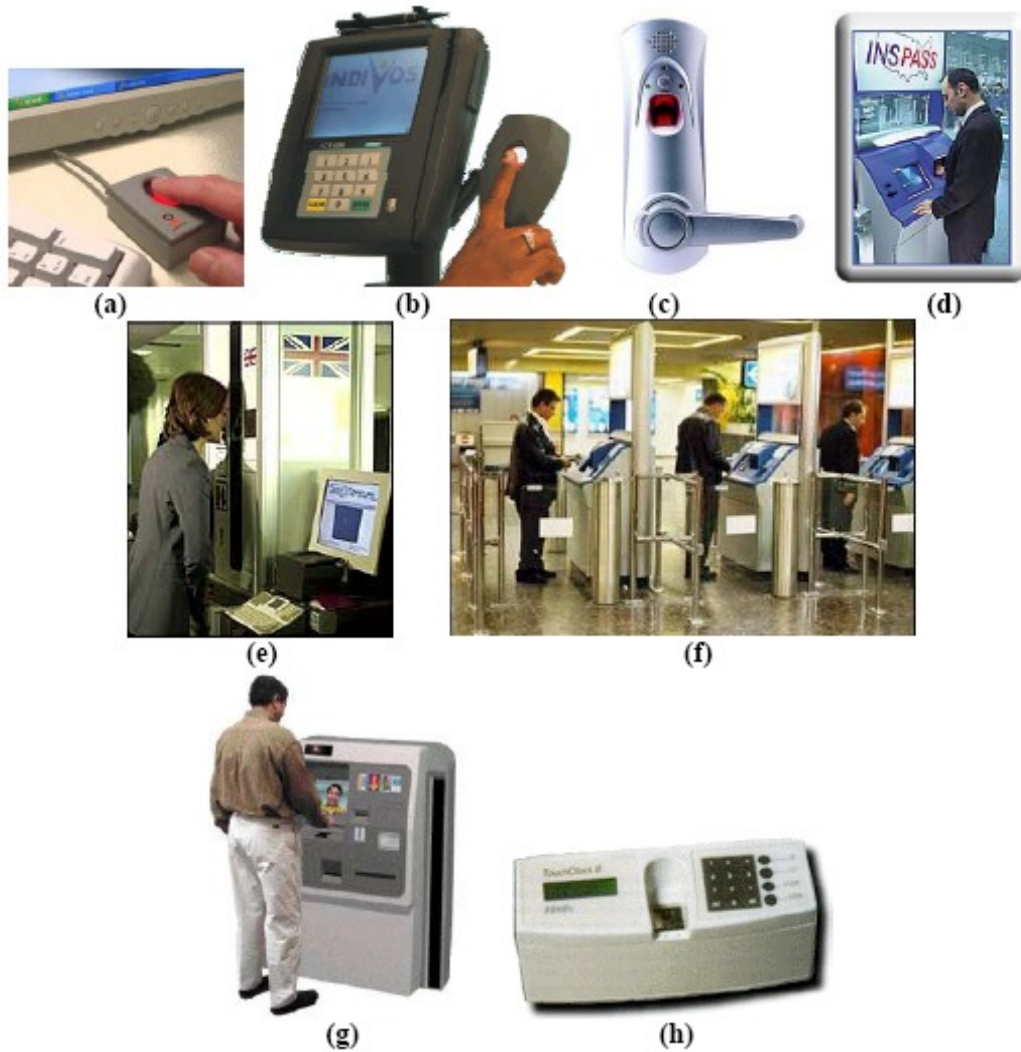
Figure 4. Examples of biometric applications. In (a), a fingerprint verification system manufactured by Digital Persona Inc. is used for computer and network login ( www.digitalpersona.com ). (b) shows a fingerprint-based point of sale (POS) terminal manufactured by Indivos Inc., that verifies the customers before charging their credit cards and speeds up payment in retail shops, restaurants and cafeterias ( www.kioskbusiness.com/JanFeb02/articles/dept3.html ). In (c), a fingerprint-based door lock manufactured by BioThentica Corp. used to restrict access to premises is shown ( www.tristarelectronics.com/newprod.php ), and (d) shows the Immigration and Naturalization Service Accelerated Service System (INSPASS), which is installed at major airports in the U.S., is based on hand geometry verification technology developed by Recognition Systems, Inc. and significantly reduces the immigration processing time ( www.panynj.gov/aviation/jfkpassframe.htm ). (e) shows a border passage system using iris recognition at London's Heathrow airport ( news.bbc.co.uk/1/hi/uk/1808187.stm ). (f) Ben Gurion airport in Tel Aviv (Israel) uses Express Card entry kiosks fitted with hand geometry systems for security and immigration ( www.airportnet.org/depts/federal/press/articles/msnbc0403.htm ). (g) The FacePass system from Viisage is used in POS verification applications like ATMs, therefore, obviating the need for PINs ( www.viisage.com/Viisage_2001.pdf ). (h) The Identix TouchClock fingerprint system is used in time and attendance applications ( www.cardsolutions.com/products/biometrics.html ).
