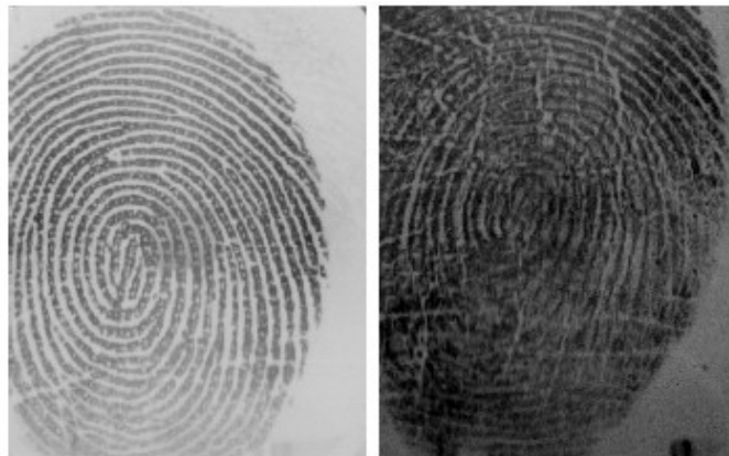
Figure 5. Effect of noisy images on a biometric system. (a) Fingerprint obtained from a user during enrollment. (b) Fingerprint obtained from the same user during verification after three months. The development of scars or cuts can result in erroneous fingerprint matching results.
